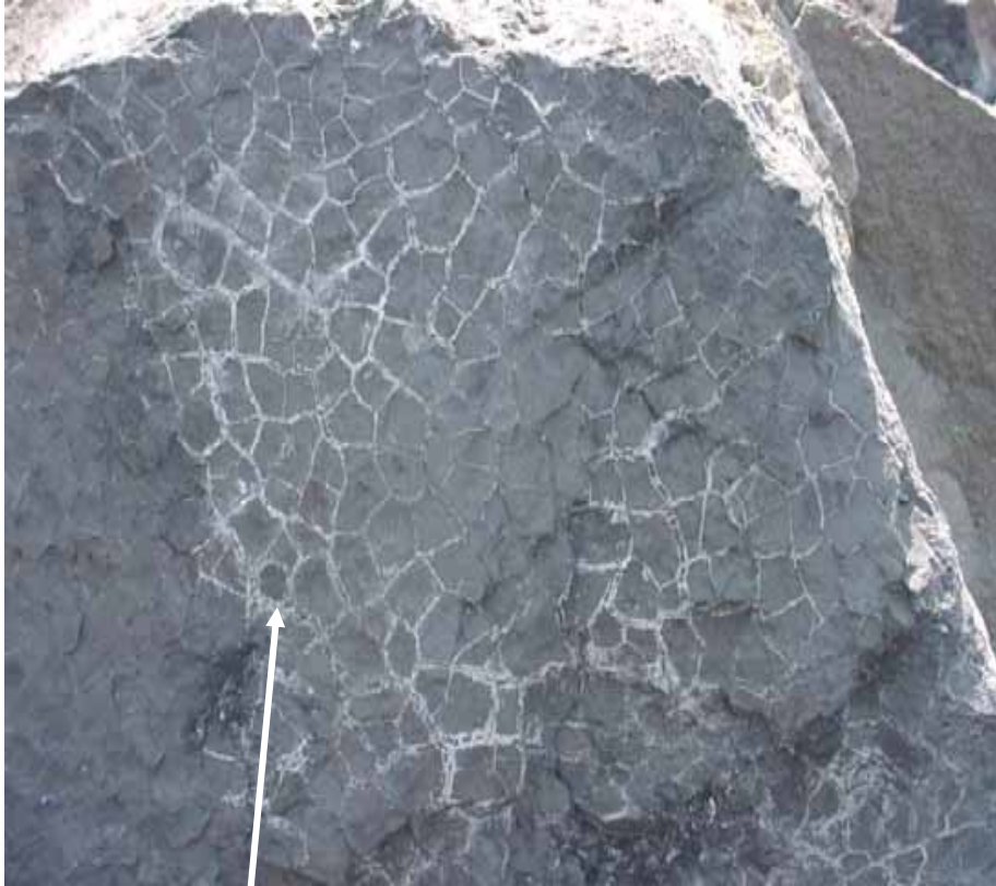
Fig1. Jhama coal showing Tortoise back structure filled up with hard rock
